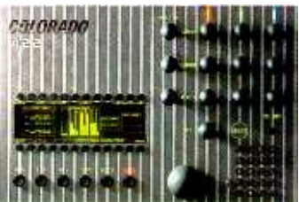
the Colorado 4:2:2 digital component color processor,
